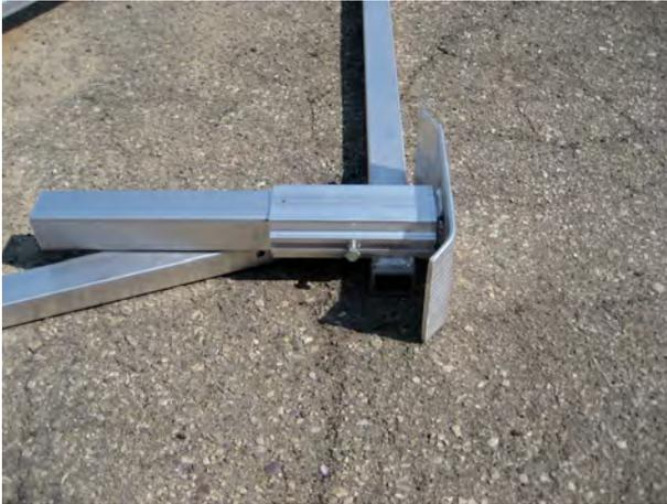
Slide the lift legs into lift side frame, as shown on the picture to the left. Tighten the legs by sliding the 3/8" square nut into the channel and tighten down using the 3/8" x 1" bolt. **Repeat this step for all four legs.**
