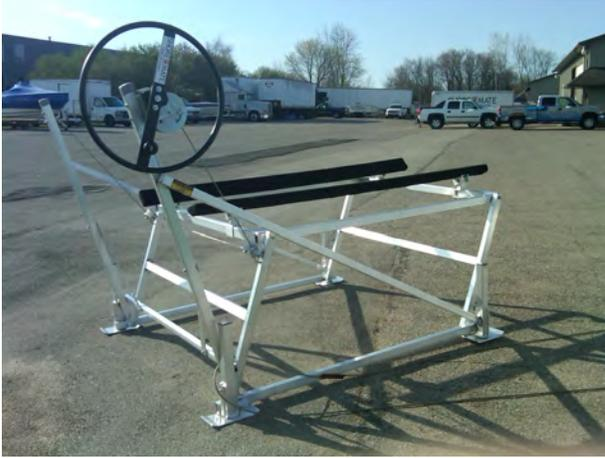
Next attach the bunks to the brackets by using the 3/8" x 3" bolts and the 3/8" wiz nuts. The bunks can swivel and should not be tightened all of the way at this point. Wait until you place your PWC on the bunks and then remove the PWC and then proceed to tighten down the bunks. The picture to the left shows what the finish product should look like.
