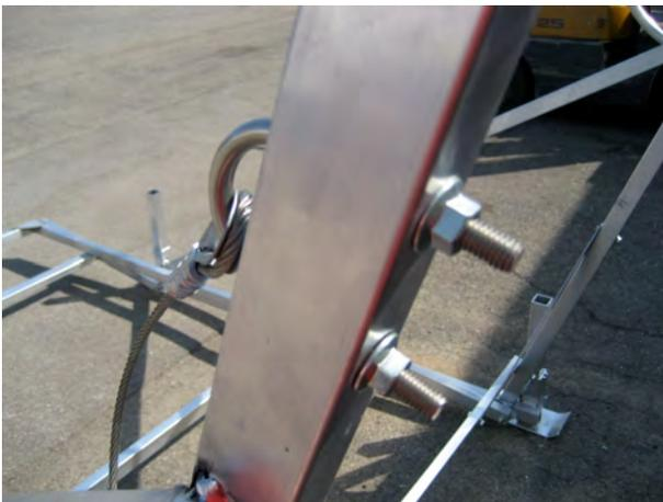
Loop the winch cable through the 3/8" round U-bolt and attach the U-bolt to the post opposite of the winch using the 3/8" wiz nuts, as shown in the picture on the left.
