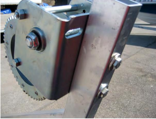
Attach the winch so that the hub is facing out. Using the 3/8" x 3-1/2" and the 3/8" winch nuts attach the winch to the upright, as shown in the picture to the left. The winch can also be placed on the opposite side by flipping it upside down
