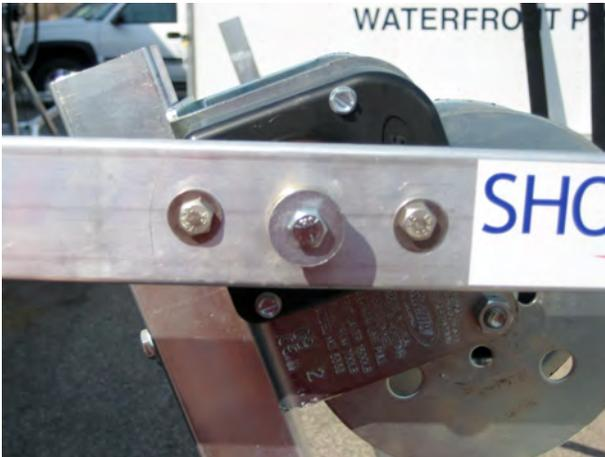
Using the wheel fastener kit attach the 24" winch wheel to the hub of the winch. The wheel fastener kit consists of the bolt, washer, spring, and spacer. Screw the bolt into the hub until the spring is compressed completely.
