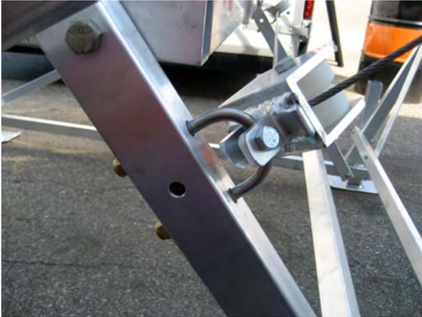
Attach the pulley brackets using the 3/8" round U-bolts. Make sure that pulley brackets are off set so that the longer part of the bracket is facing inwards. Attach the u-bolt using the 3/8" nyloc nuts. Repeat this step for the other pulley.
