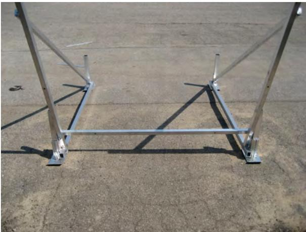
After attaching the front bottom beam the lift should look like the picture on the left.
