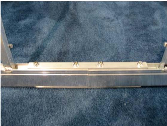
The picture on the left shows what the splice kit should look like when finished. This picture is taken from the outside of the rail looking in. Make sure that these nuts are tight so that the canopy doesn't sag.
