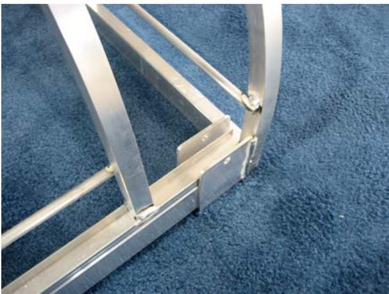
Place the canopy rails into the canopy ends as shown in the picture on the left. It works best to wait and put the middle rails into the end piece after this step.
