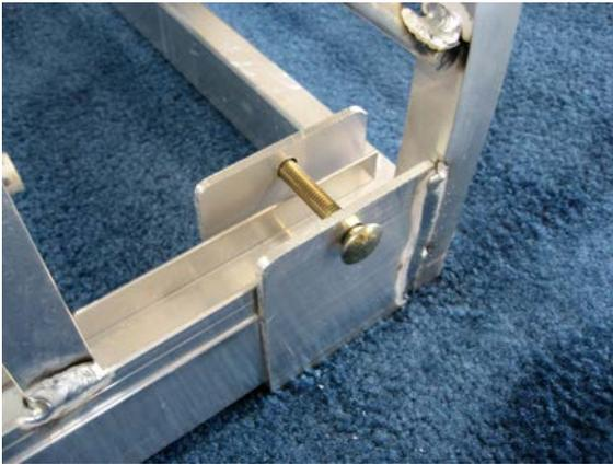
Once the canopy ends are attached, use (2) 3/8" x 2-1/2" Carriage Bolts and (2) 3/8" Flange Nuts to attach the canopy end on the bottom, as shown in the picture on the left. Repeat these steps for the other canopy end!
