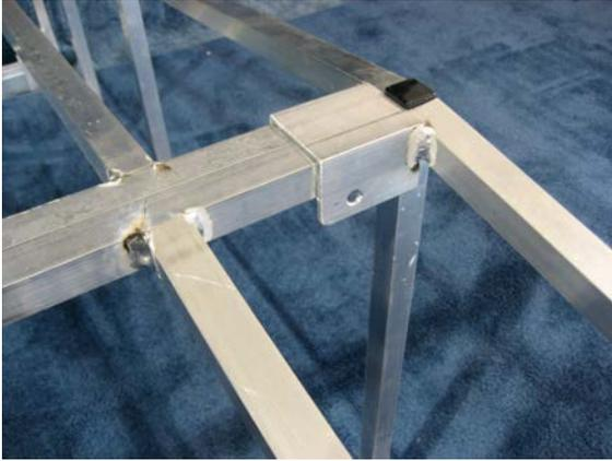
Once the two end rails are attached to the canopies end then it is time to place the middle rail into the canopy end, as shown in the picture on the left. Use (1) 3/8" x 2-1/2" bolt and (1) 3/8" Flange Nut to tighten the canopy end.
