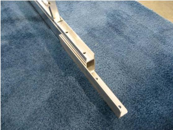
Take the angle bracket and make sure that it is facing inward. Line the bracket up as shown in the pictures on the left.
