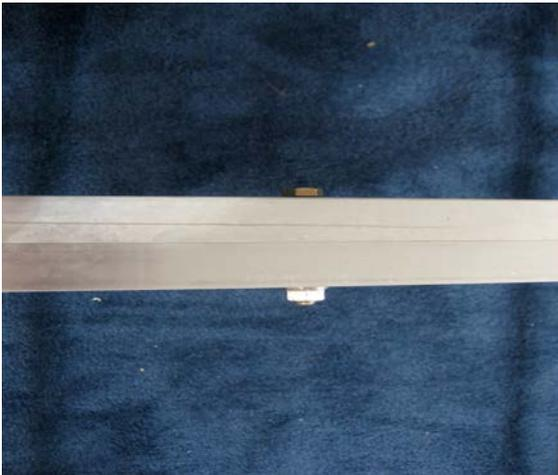
Use the 3/8" x 2-1/2" Bolts and the 3/8" Flange Nuts to attach the middle sections of the canopy together as shown in the picture on the left. Do this for both halves of the canopies.
