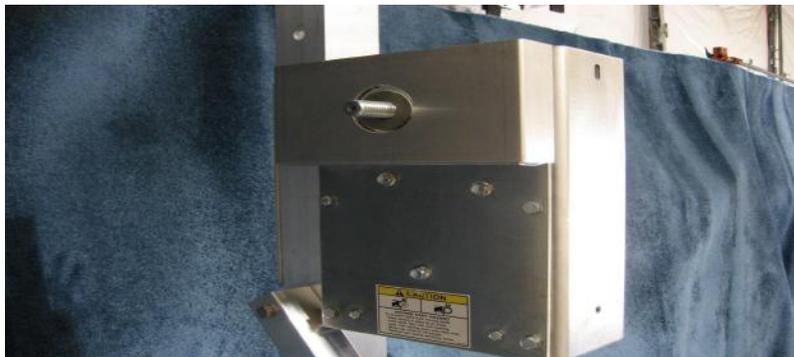
For this step you will need the 42" winch wheel as well as the spinner knob, 3/8" fender washer, and a 5/16" x 2" hex head bolt.
