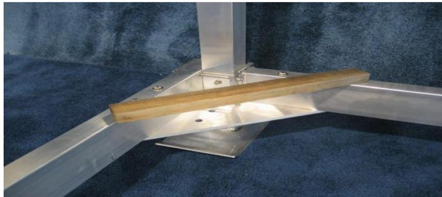
The front and rear bed beam is shown here to the left. These beams run right to left across the lift and not front to back. The rear bed beam has two cables in the beam and is placed opposite of the winch. The front bed beam has one cable in the beam and is placed alongside the winch running right to left.
