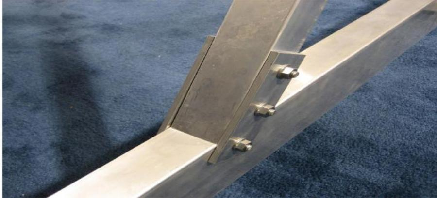
Next, take the corner post bracket and slide it over the top of the column. Slide the diagonal brace so that the holes of the diagonal brace and the corner post bracket align, and using the 1/2" x 6" hex head bolt and flange nut, attach the diagonal brace to the corner post bracket. Repeat this step for the other
