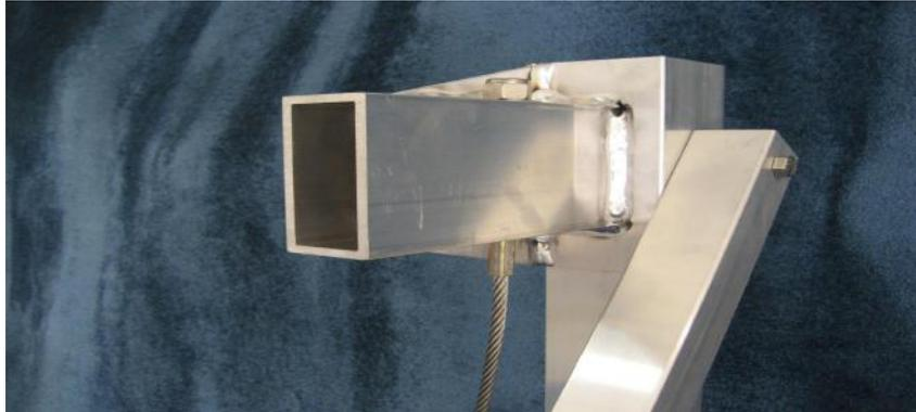
This picture shows how the cables that run down are connected to the corner plate. Here you can see the washer as well as the nylock nut. These cables are tightened as far as possible. **Do not tighten these cables at this time!**
